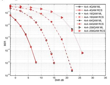
Figure 8 ML against RCS-ML decoding performance comparison for the QO-STBC MIMO system with different QAM constellation size,  $n_T = 4 \times n_R = 1$  antennas
