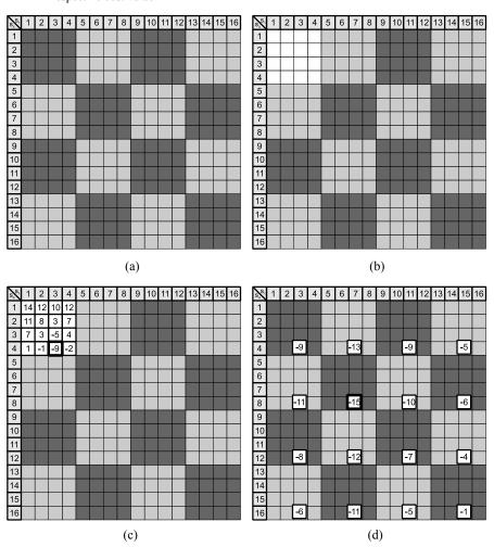
Figure 6 Example of RCS decoding and 16-QAM, (a) search space divided in clusters (b) first *cluster* to be explored (c) cost for each pair  $(s_1, s_4)$  inside first cluster (d) local minima with respective cost value
