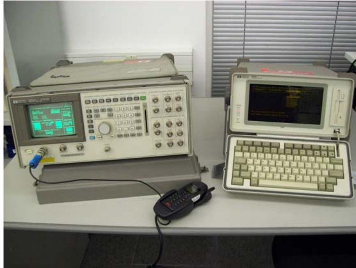
Figure 4. HP8922H connected to HP37900D to analyze GSM physical layer signaling
