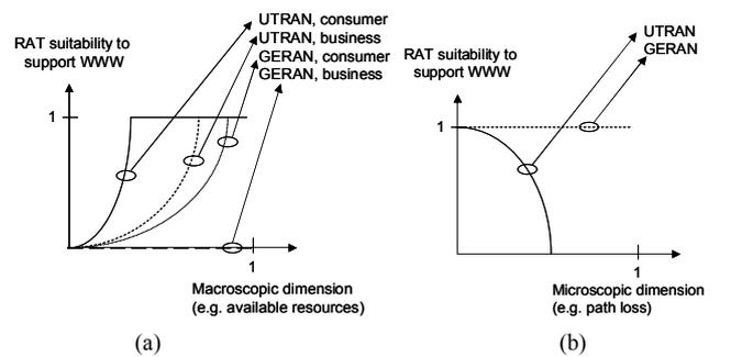
Figure 2. Suitability as a function of the macroscopic (a) and microscopic (b) dimensions.
