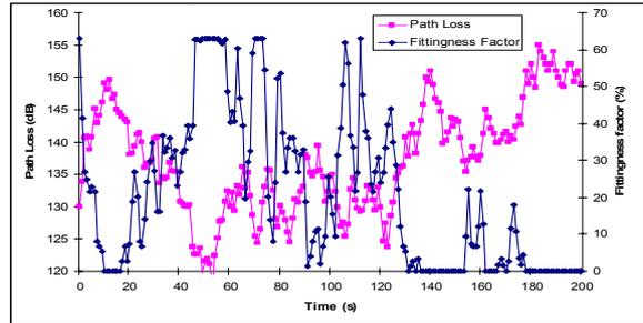
Figure 3. Example of time evolution of the path loss and the fittingness factor for a consumer interactive user in the central cell of UTRAN
